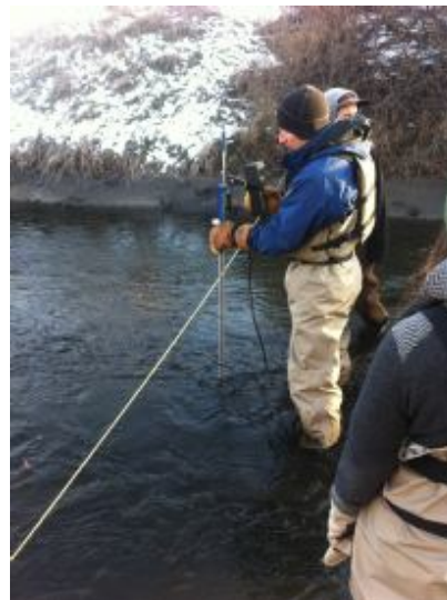
Figure 5. Stream flow measurement using a Flow Tracker in Shingle Creek, Minneapolis, Minnesota.
