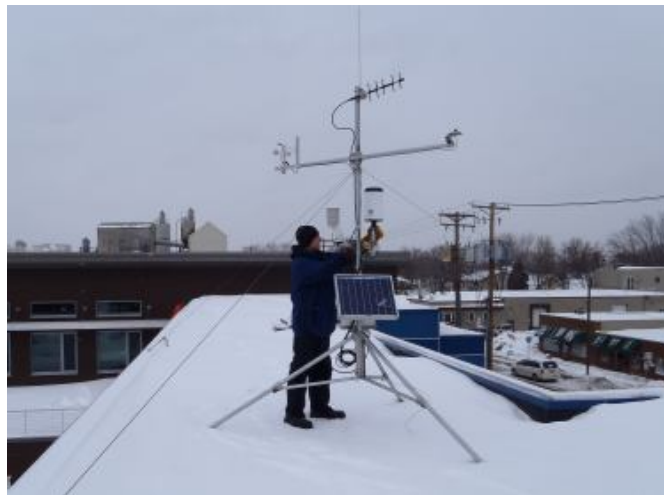
Figure 1. An example of Automated Weather Station at the Roof Top of MWMO Stormwater Park and Learning Center building, Minneapolis, Minnesota, USA.
