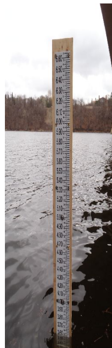
Figure 4: River Staff Gauge to Manually Monitor River Levels.
