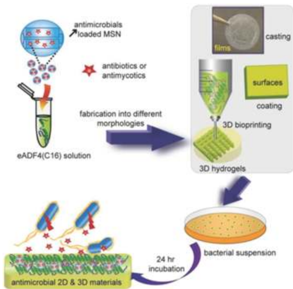
Fig. 9. Schematic fabrication process for hybrid scaffolds composed of recombinant spider silk and silica loaded with antimycotics and antibiotics. Reproduced from Kumari et al., 2020.
